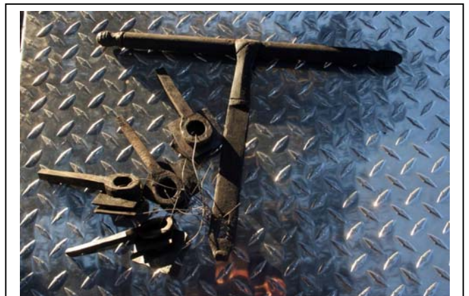
William “Bill” Martini’s reproduction of a Mission era slide bolt for the new Gift Shop Manager’s office door. Bill used borax to fuse the arm of the latch to the slide bolt. The “eyelet” elements serve as fasteners for the slide bolt pictured. Photo © Ruben G. Mendoza, 2007.
